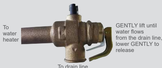
How to operate the easing gear
